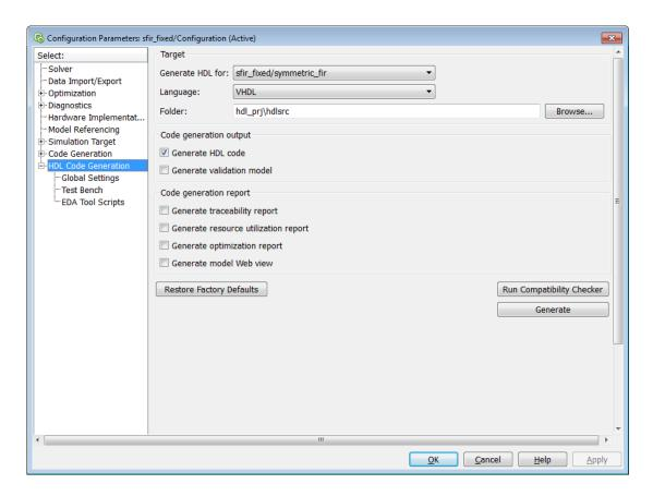
The **HDL Code Generation** pane contains top-level options and buttons that control the HDL code generation process. Several other categories of options are available under the **HDL Code** entry. This exercise uses a small subset of these options, leaving the others at their default settings.
