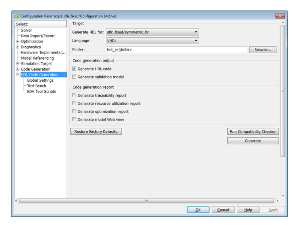
The following figure shows the top-level **HDL Code Generation** options pane in the Model Explorer.
