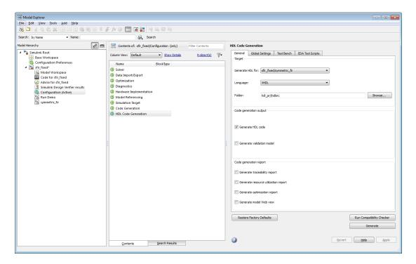
In the code generation exercises that follow, you use the Configuration Parameters dialog box to view and set HDL Coder options and controls. The exercises use the <code>sfir\_fixed</code> model (see "The sfir\_fixed Model" on page 3-16) in basic code generation and verification steps.
